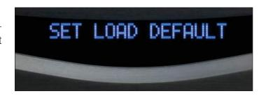
By pressing « SET » mode, access SET LOAD DEFAULT is given. On second raw is shown flashing NO. By turning volume knob, status changes and it is displayed YES.
