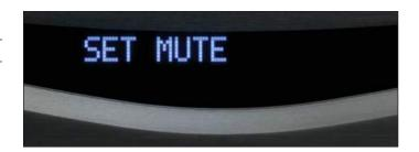
By pressing « SET » mode, access SET MUTE is given. On second raw TOTAL is shown flashing (-90 dB). By turning volume knob, MUTE status changes and it is displayed (-30 dB).
