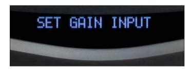
Further confirming SET, gain of selected input flashes and it can be increased or decreased, by 1 dB steps, up to 6 dB maximum, in order to equalize levels.
