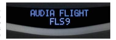
First line on display shows selected input (# 1 by default), second line shows volume level in dB of output signal (- 90 dB, by default, the lowest possible).
