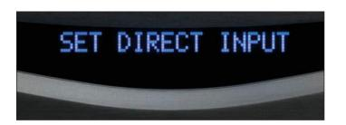
By pressing « SET » mode, access SET DIRECT INPUT is given. On second raw is shown the selected input. By turning volume knob, input changes and it is displayed.
